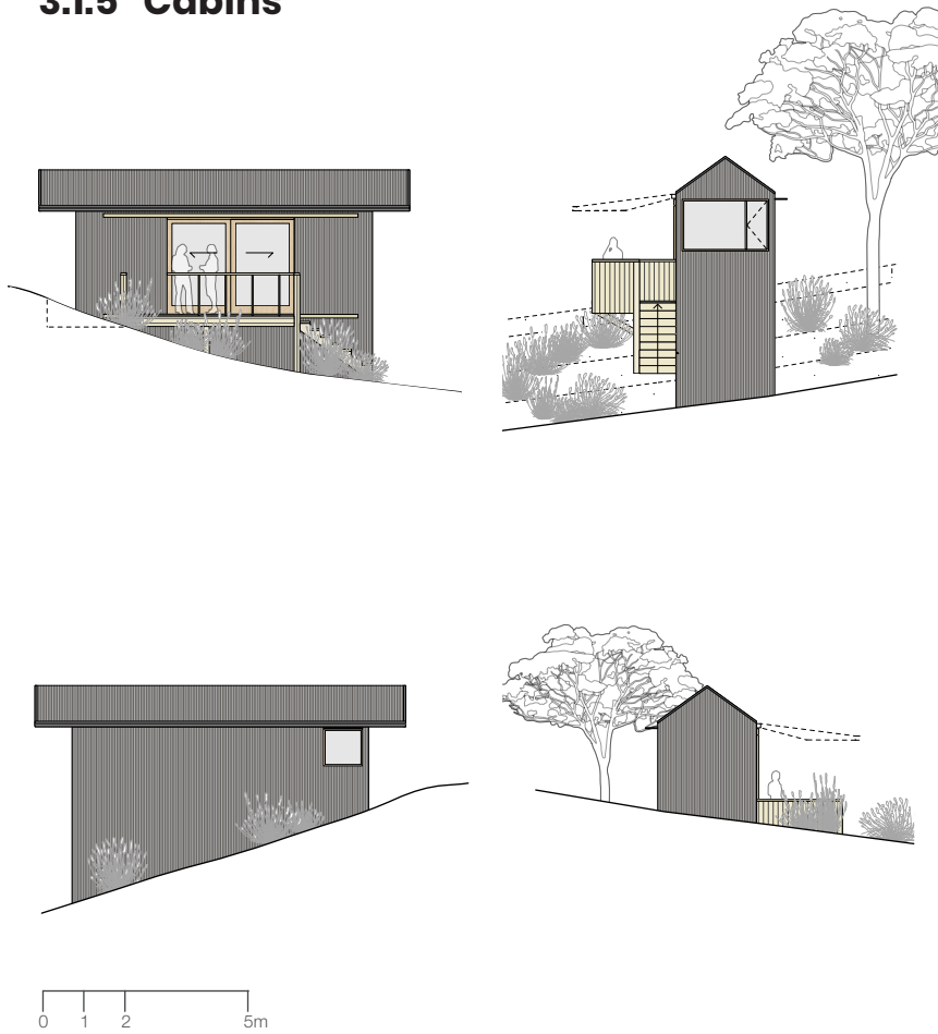
Figure 3.33 Compact cabin elevations
